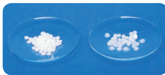
Figure 9.11 Deliquescence in Sodium hydroxide
